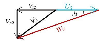
$$egin{aligned} eta_2&=15^0\ V_{t2}&=-(W_2 imes Coseta_2-U_2)\ W_2&=W_1 imes K\ 0&< K<1 \end{aligned}$$
